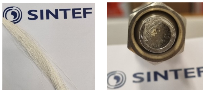
Figure 11. PPO hollow fibers and head of a module with 10 HF with a length of 30 cm
